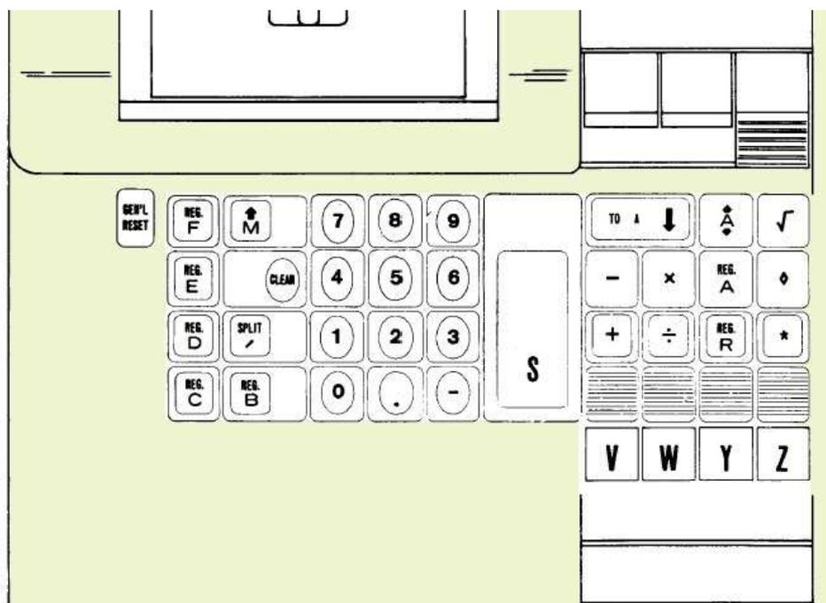
Fig. 3. Programma 101 keyboard. (Courtesy of Olivetti Underwood Corporation.)
